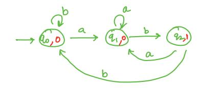
$$\begin{array}{c} ab \ a \ ab b b a b \\ q_0 \xrightarrow{a} q_1 \xrightarrow{b} q_2 \xrightarrow{a} q_1 \xrightarrow{a} q_1 \xrightarrow{b} q_2 \xrightarrow{b} q_2 \xrightarrow{b} q_0 \xrightarrow{b} q_0 \xrightarrow{a} q_1 0 \\ 0 & 0 & 1 & 0 & 0 & 1 \\ 0 & 0 & 1 & 0 & 0 & 1 \\ q_{21} \end{array}$$
